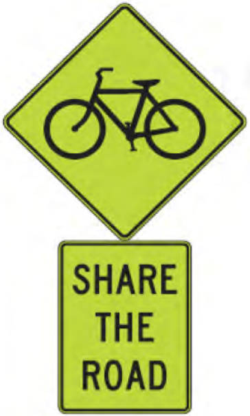
Image D-1 “Share the Road” Sign Assembly (W11-1 + W16-1P)
