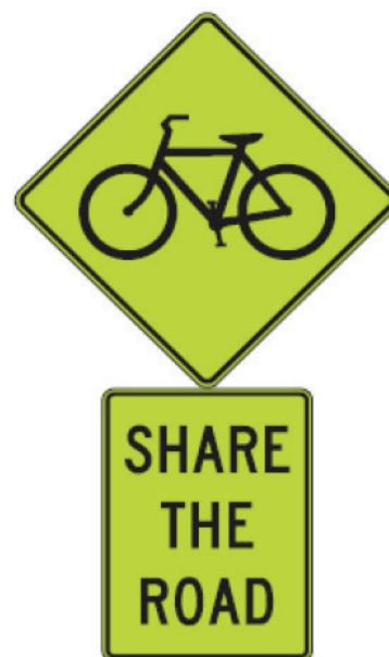
Image C-1 “Share the Road” sign assembly (W11-1 + W16-1P)
