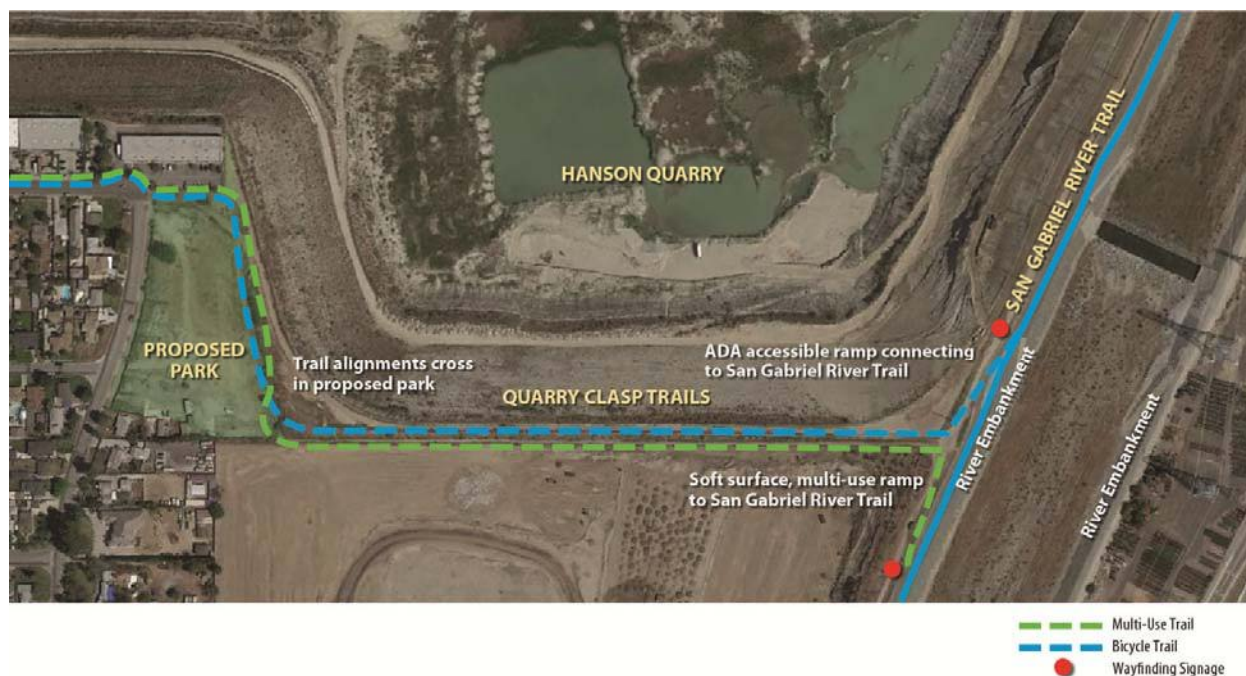
Fig. 19. Proposed trail alignments along the proposed Quarry Clasp Park and quarry spine on the Rio Hondo-San Gabriel River connection. Two ADA ramps on the levee will accommodate a soft trail and a Class I bicycle path up to the existing Class I bicycle path at the top.
